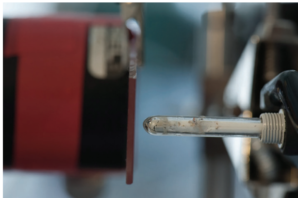
FIG. 2: Photograph of the plasma probe ~2mm away from the treatment surface (ITO-coated glass) with plasma turned off
